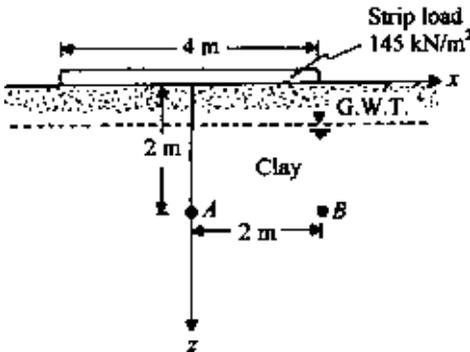
Figure 4.17 Uniform vertical strip load on ground surface.
