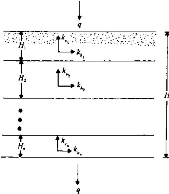
Figure 5.15 Flow in vertical direction in stratified soil.
