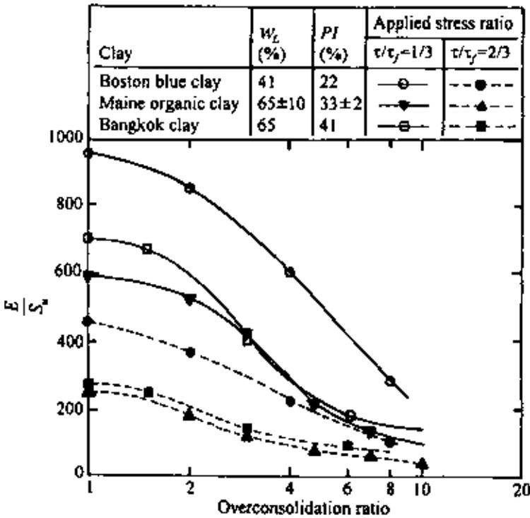
Figure 8.2 Relation between  $E/S_u$  and overconsolidation ratio from consolidated undrained tests on three clays determined from  $CK_oU$  type direct shear tests (after D'Appolonia et al., 1971).
