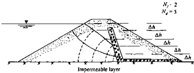
Figure 5.62 Typical flow net for an earth dam with chimney drain.
