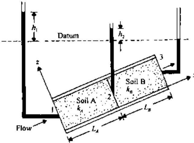
Figure 5.25 One-directional flow through two layers of soil.
