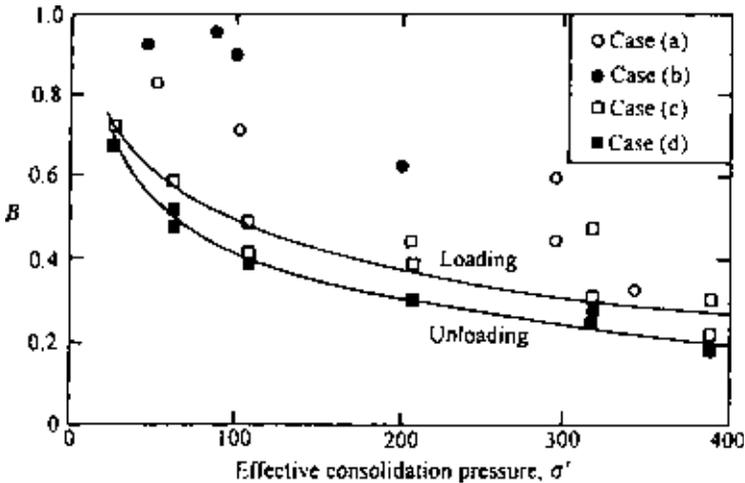
Figure 4.7 Dependence of  $B$  values on level of isotropic consolidation stress (varved clay) for (a) regular triaxial specimens before shearing, (b) regular triaxial specimens after shearing, (c) special series of  $B$  tests on one single specimen in loading, and (d) special series of  $B$  tests on one single specimen in unloading (after Eigenbrod and Burak, 1990).
