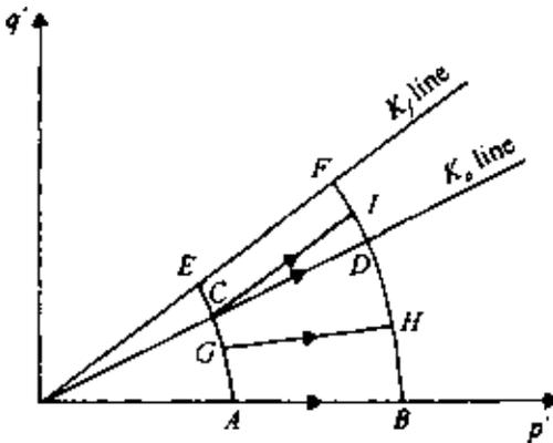
Figure 8.24 Volume change between two points of a  $p'$  versus  $q'$  plot.
