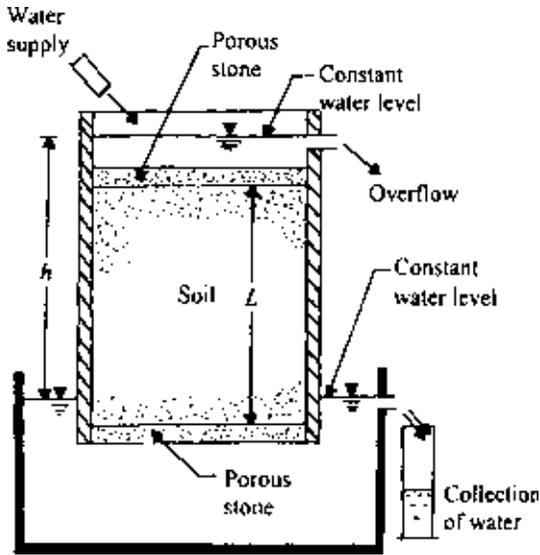
Figure 5.4 Constant-head laboratory permeability test.
