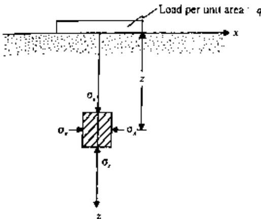
Figure 4.16 Estimation of excess pore water pressure in saturated soil below the centerline of a flexible strip loading (undrained condition).
