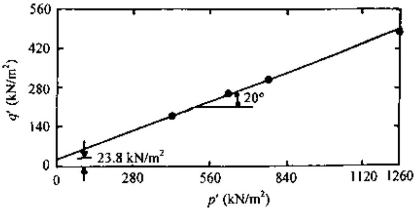
Figure 7.45 Plot of  $q'$  versus  $p'$  diagram.
