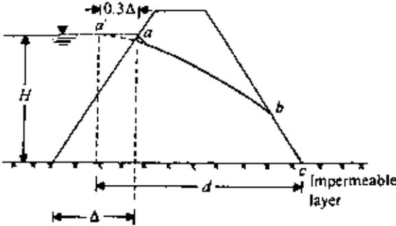
Figure 5.51 Modified distance  $d$  for use in Eq. (5.184).
