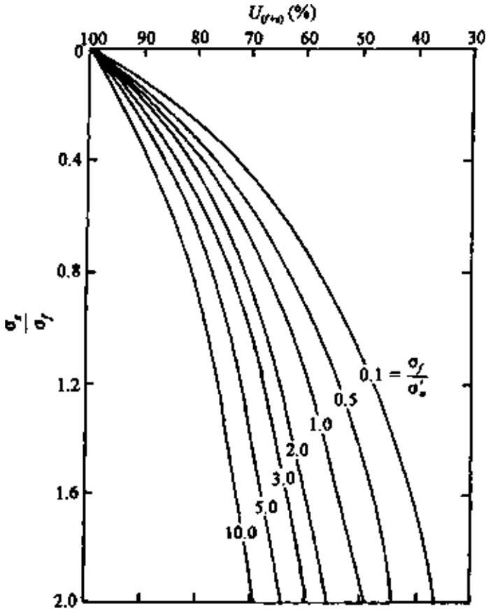
Figure 8.29 Variation of  $U_{(f+s)}$  with  $\sigma_v/\sigma'_f$  and  $\sigma'_h/\sigma'_v$ .
