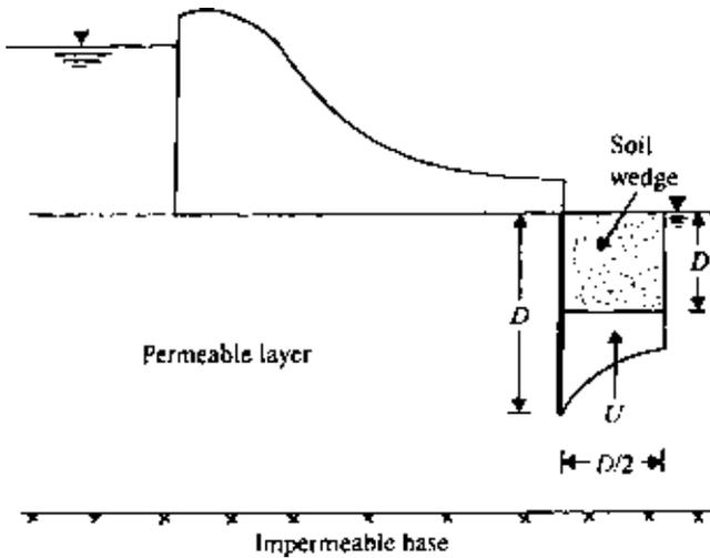
Figure 5.43 Safety against piping under a dam.
