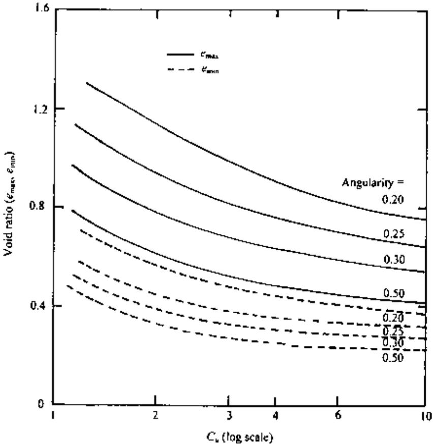
Figure 1.35 Youd's recommended variation of  $e_{max}$  and  $e_{min}$  with angularity and  $C_u$ .
