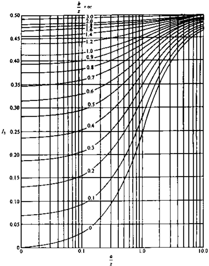
Figure 3.15 Influence factors for embankment load (after Osterberg, 1957).
