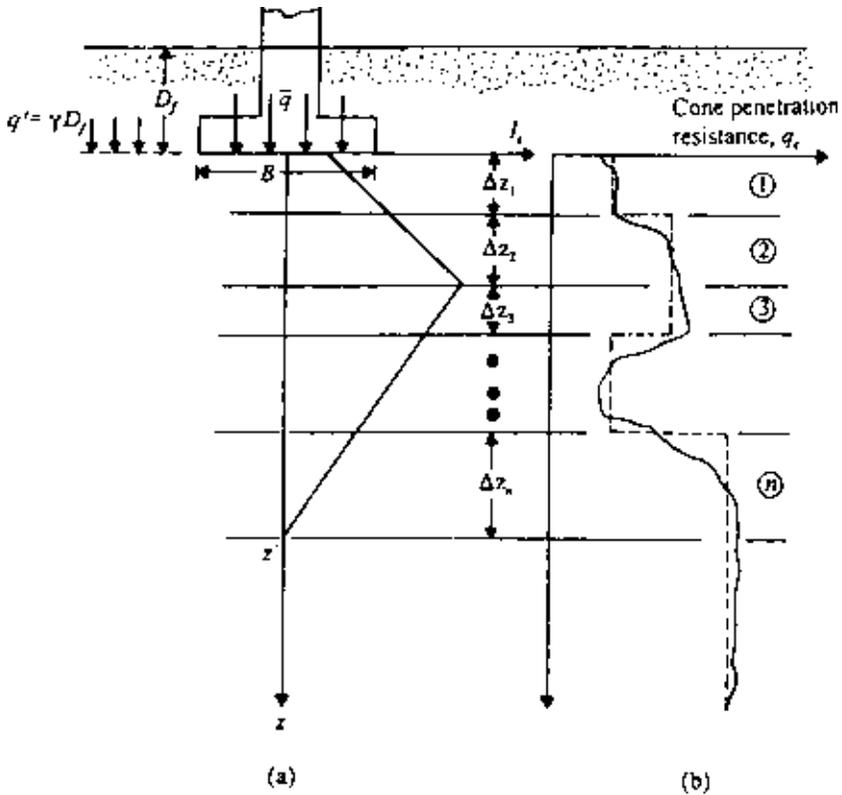
Figure 8.12 Calculation of  $S_e$  from strain influence factor.
