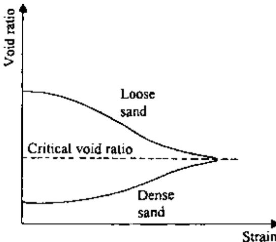
Figure 7.11 Definition of critical void ratio.
