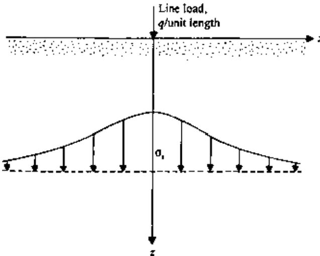
Figure 2.11 Stress at a point due to a line load.
