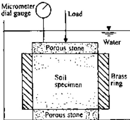
Figure 6.13 Consolidometer.
