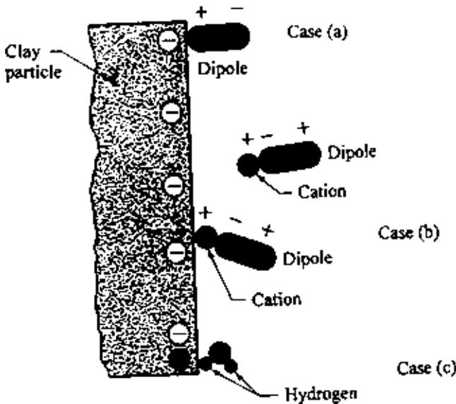
Figure 1.7 Dipolar water molecules in diffuse double layer.
