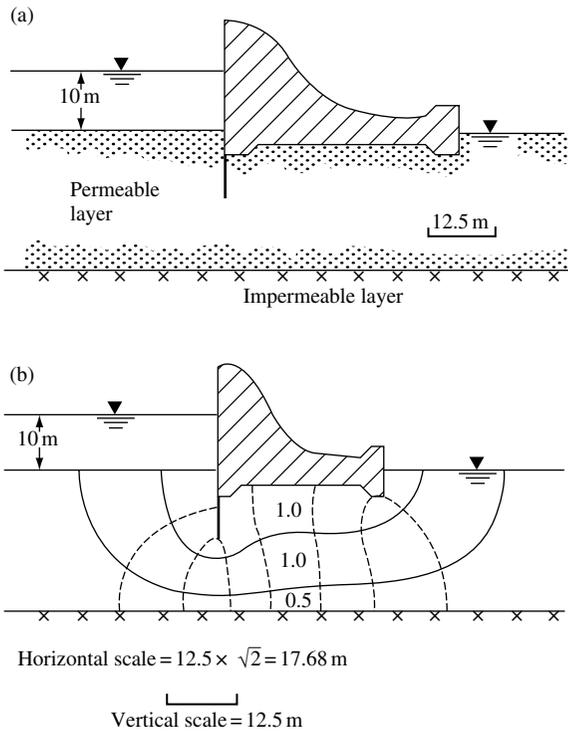
Figure 5.31 Construction of flow net under a dam.
