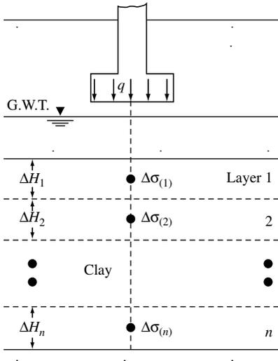
Figure 8.15 Calculation of consolidation settlement—method B.
