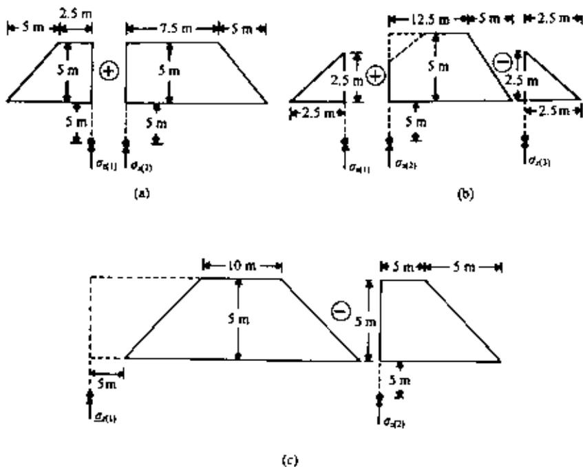
Figure 3.17 Calculation of stress increase at A, B, and C (Not to scale).
