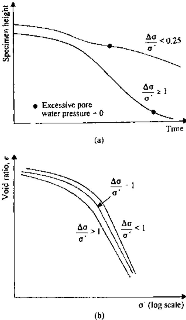
Figure 6.19 Effect of load-increment ratio.
