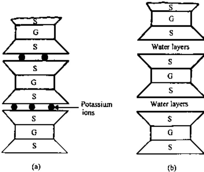
Figure 1.4 Symbolic structures of (a) illite and (b) montmorillonite.
