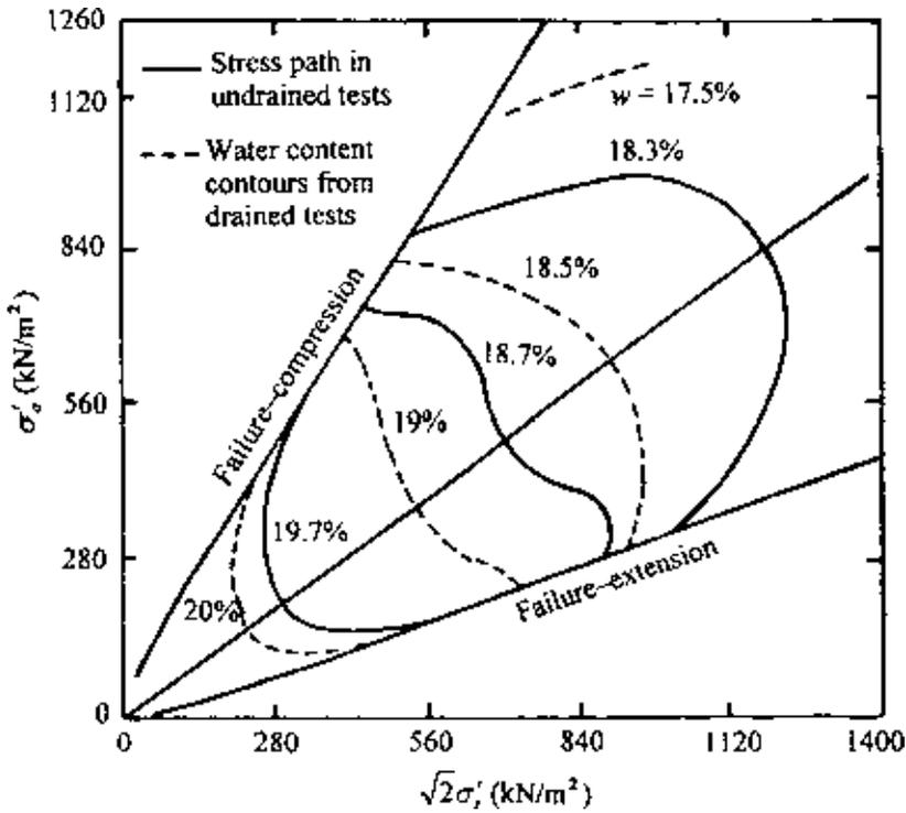
Figure 7.55 Weald clay—overconsolidated; maximum consolidation pressure = 828 kN/m<sup>2</sup> (after Henkel, 1960).
