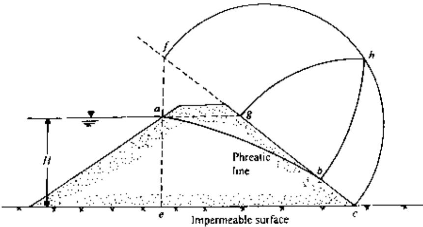
Figure 5.50 Graphical construction for Schaffernak's solution.
