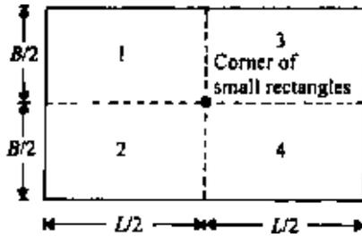
Figure 3.28 Determination of settlement at the center of a rectangular area of dimensions  $L \times B$ .
