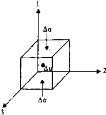
Figure 4.8 Saturated soil element under uniaxial stress increment.
