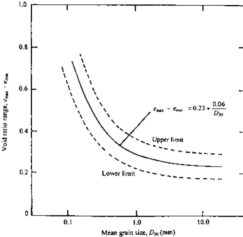
Figure 1.37 Plot of  $e_{\max} - e_{\min}$  versus the mean grain size.
