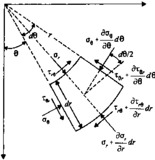
Figure 2.7 Derivation of static equilibrium equation for two-dimensional problem in polar coordinates.
