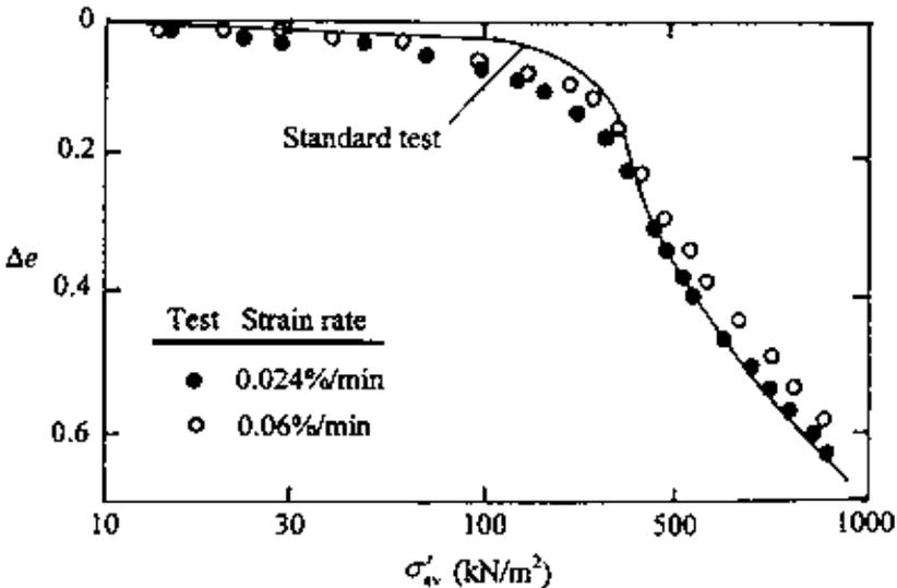
Figure 6.34 CRS tests on Massena clay—plot of  $\Delta e$  versus  $\sigma'_{av}$  (after Smith and Wahls, 1969).
