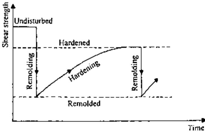
Figure 7.63 Regained strength of a partially thixotropic material.
