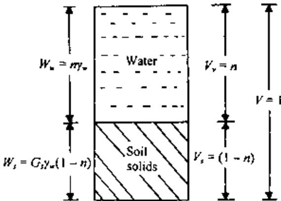
Figure 1.34 Weight–volume relationship for saturated soil with  $V = 1$ .
