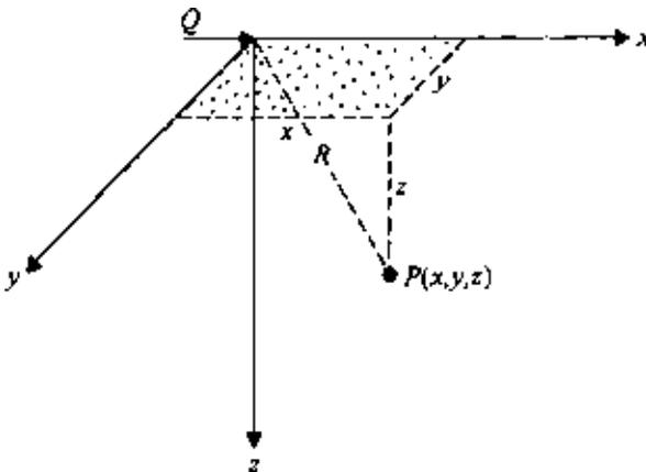
Figure 3.20 Horizontal point load on the surface.
