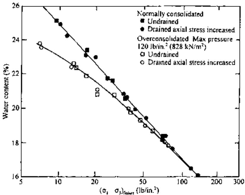
Figure 7.50 Water content versus  $(\sigma_1 - \sigma_3)_{failure}$  for Weald clay—compression tests [Note: 1 lb/in<sup>2</sup> = 6.9 kN/m<sup>2</sup>; after Henkel (1960)].
