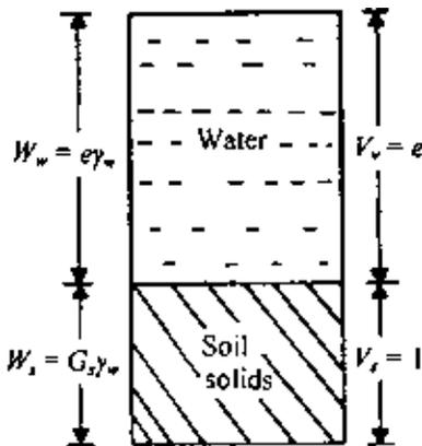
Figure 1.32 Weight–volume relation for saturated soil with  $V_s = 1$ .
