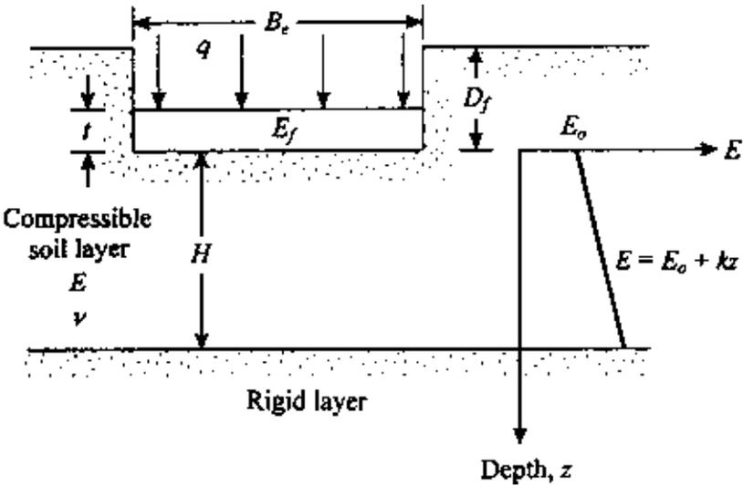
Figure 8.7 Improved equation for calculating elastic settlement—general parameters.
