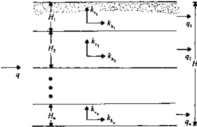
Figure 5.14 Flow in horizontal direction in stratified soil.
