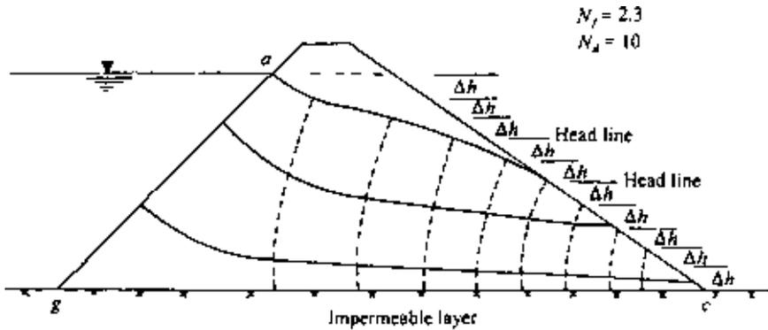
Figure 5.60 Flow net construction for an earth dam.
