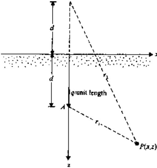
Figure 3.5 Vertical line load inside a semi-infinite mass.
