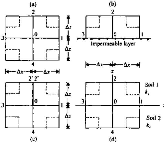
Figure 5.37 Numerical analysis of seepage.
