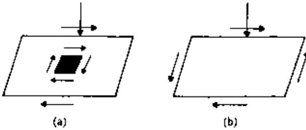
Figure 7.6 (a) Simple shear and (b) Pure shear.
