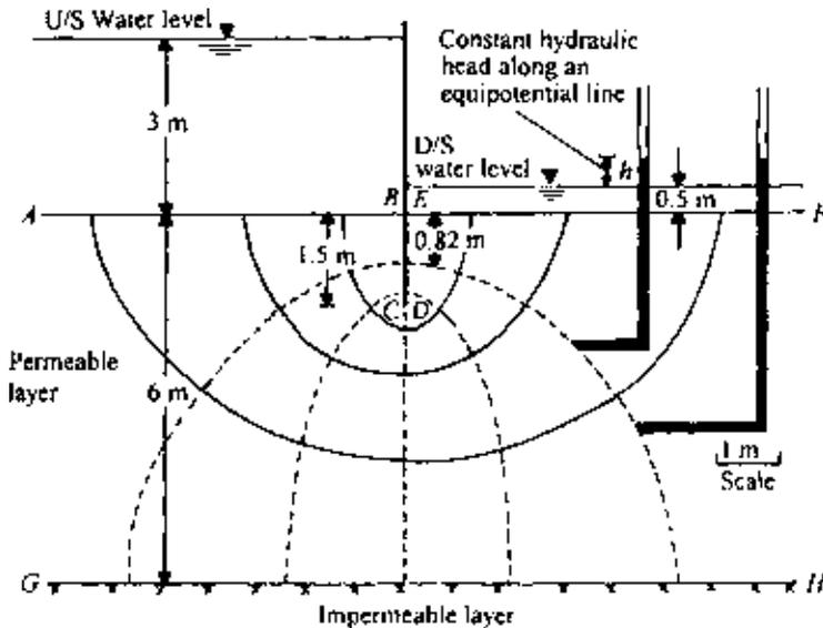
Figure 5.26 Flow net around a single row of sheet pile structures.
