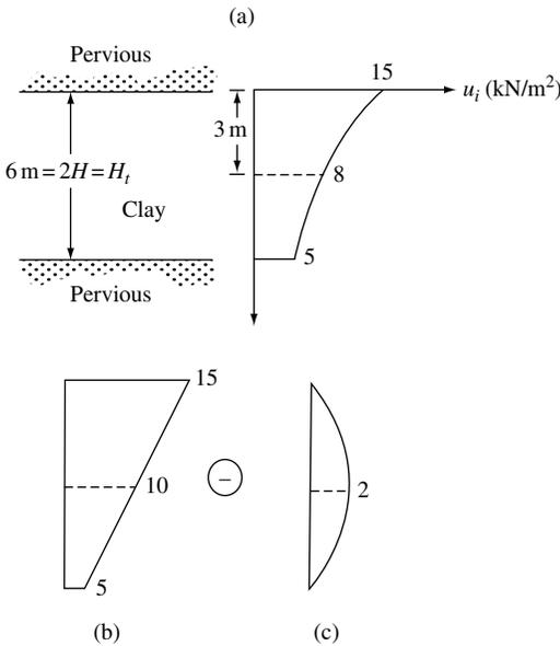
Figure 6.6 Calculation of average degree of consolidation ( $T_v = 0.3$ ).
