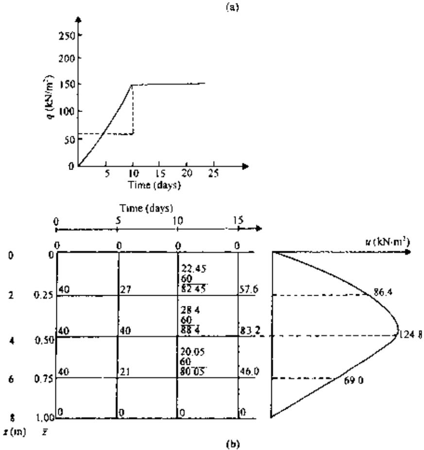
Figure 6.12 Numerical solution for ramp loading.
