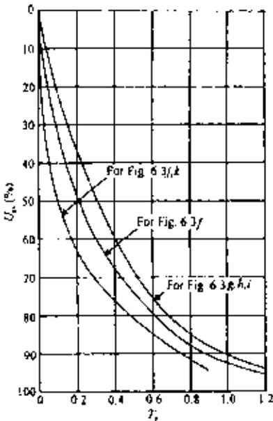
Figure 6.5 Variation of  $U_{av}$  with  $T_v$  for initial excess pore water pressure diagrams shown in Figure 6.3.
