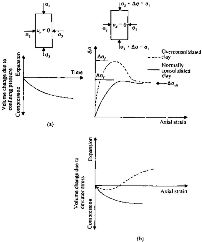
Figure 7.18 Consolidated drained triaxial test in clay (a) Application of confining pressure and (b) Application of deviator stress.
