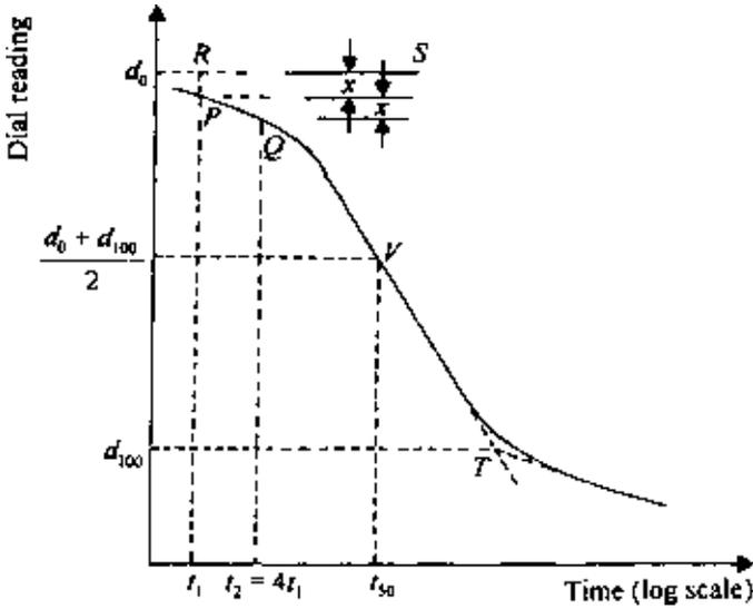
Figure 6.24 Logarithm-of-time method for determination of  $C_v$ .
