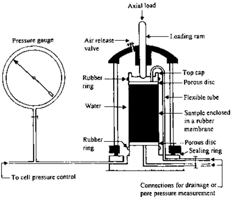
Figure 7.7 Triaxial test equipment (after Bishop and Bjerrum, 1960).
