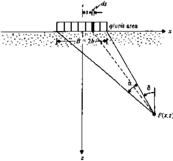
Figure 3.9 Uniform vertical loading on an infinite strip.
