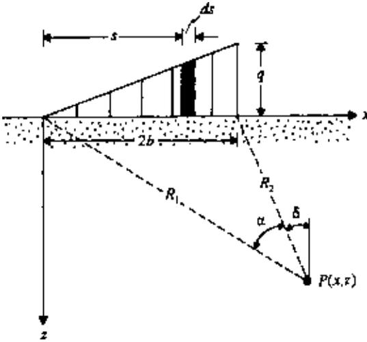
Figure 3.13 Linearly increasing vertical loading on an infinite strip.
