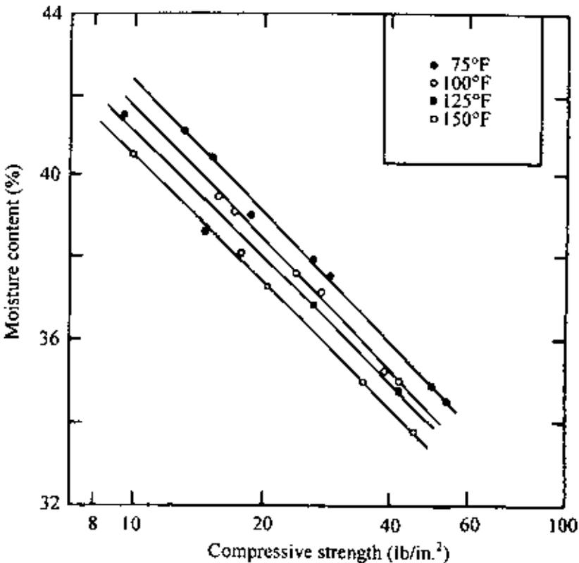
Figure 7.35 Unconfined compression strength of kaolinite—effect of temperature (After Sherif and Burrous, 1969). (Note: 1 lb/in.<sup>2</sup> = 6.9 kN/m<sup>2</sup>.)
