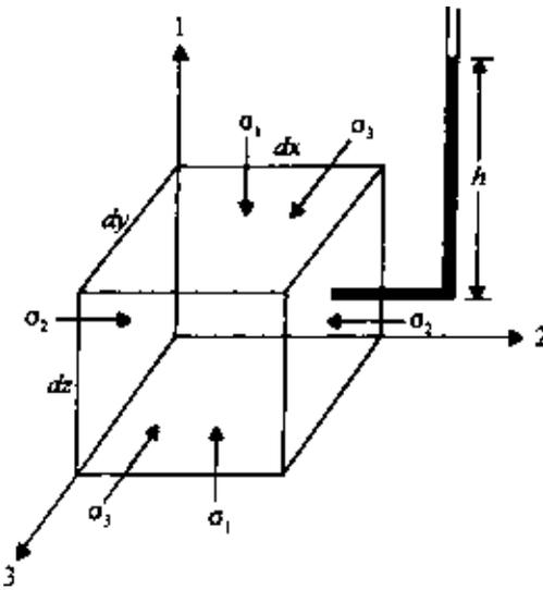
Figure 4.2 Normal total stresses in a soil mass.
