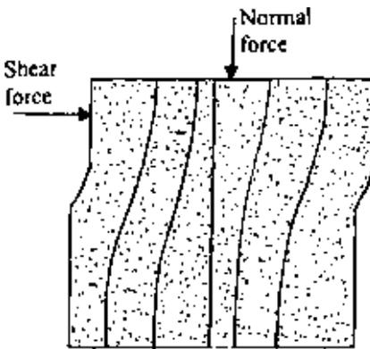
Figure 7.5 Unequal stress distribution in direct shear equipment.
