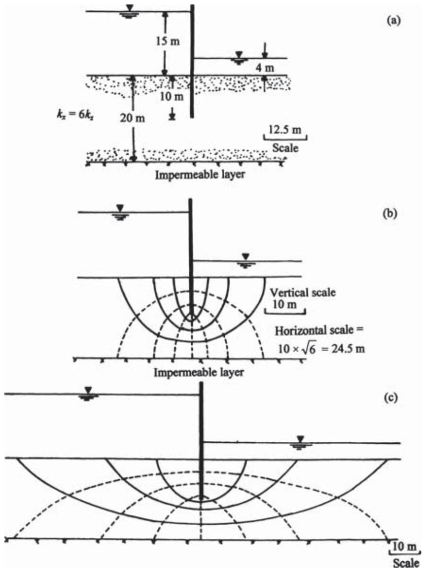
Figure 5.32 Flow net construction in anisotropic soil.
