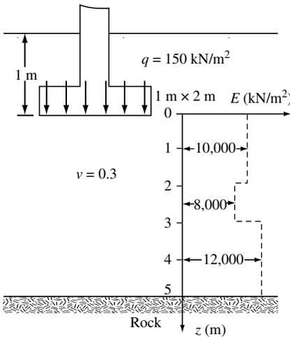
Figure 8.5 Elastic settlement for a rigid shallow foundation.
