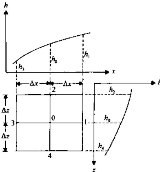
Figure 5.36 Hydraulic heads for flow in a region.
