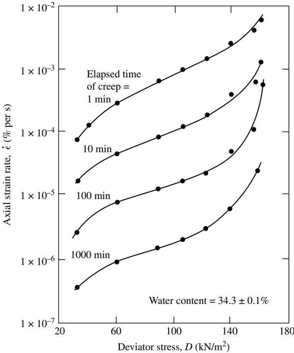
Figure 7.79 Variation of strain rate with deviator stress for undrained creep of remolded illite (after Mitchell *et al.*, 1969).
