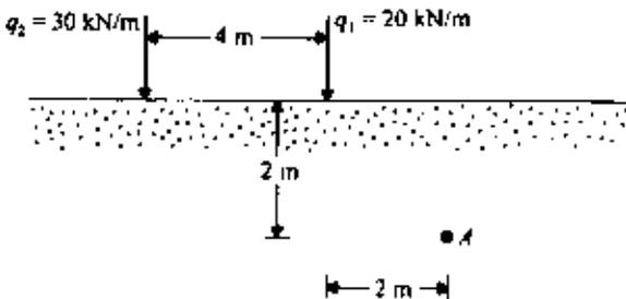
Figure 3.3 Two line loads acting on the surface.
