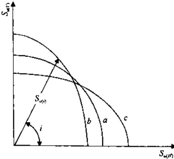
Figure 7.57 Directional variation of undrained strength of clay.
