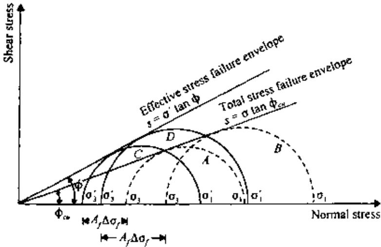
Figure 7.25 Consolidated undrained test results—normally consolidated clay.
