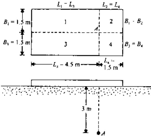
Figure 3.27 Distributed load on a flexible rectangular area.
