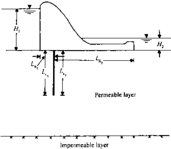
Figure 5.41 Calculation of weighted creep distance.
