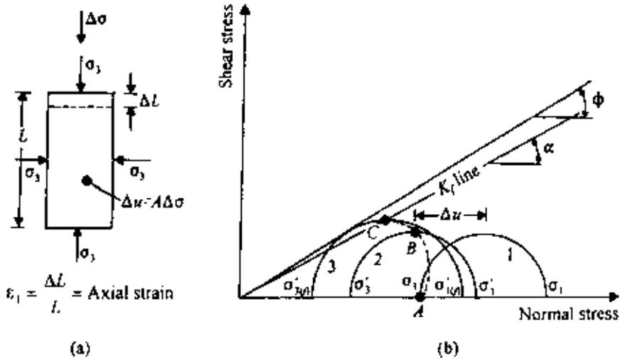
Figure 7.41 Stress path for consolidated undrained triaxial test.
