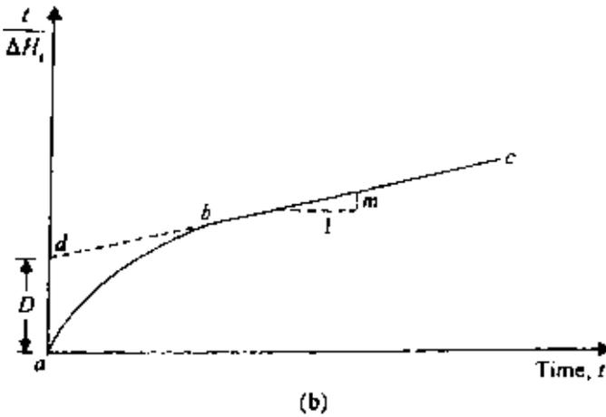
Figure 6.27 Rectangular hyperbola method for determination of  $C_v$ .
