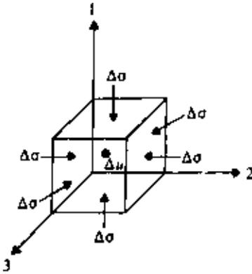
Figure 4.3 Soil element under isotropic stress application.
