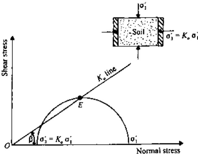
Figure 8.21 Determination of the slope of  $K_o$  line.
