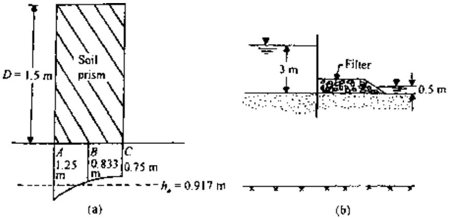
Figure 5.44 Factor of safety calculation by Terzaghi's method.
