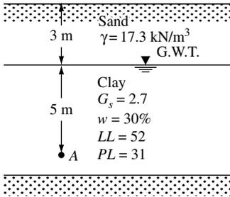
Figure 7.71 Undrained shear strength of a clay deposit.
