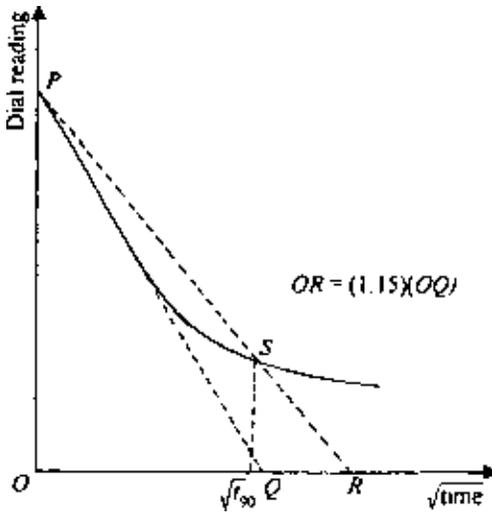
Figure 6.25 Square-root-of-time method for determination of  $C_v$ .
