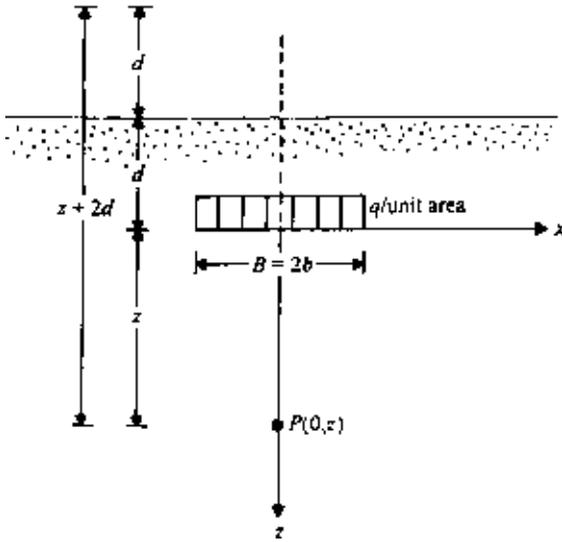
Figure 3.10 Strip load inside a semi-infinite mass.
