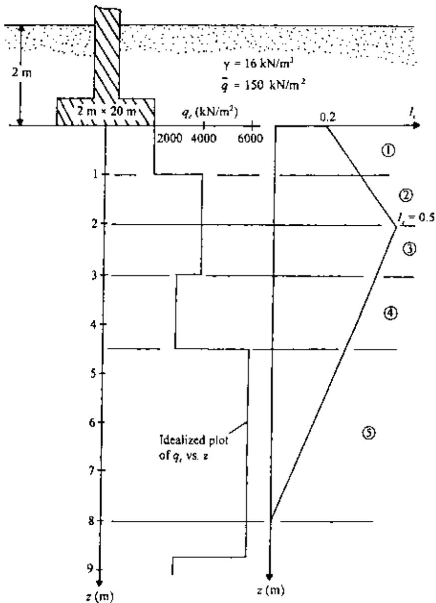
Figure 8.13 Settlement calculation under a pier foundation.
